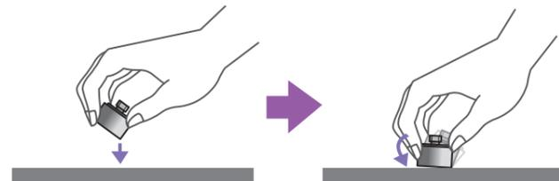
まず、一方の角をそと対象物に当てます。First, place one corner of the holder on the object to be measured.
