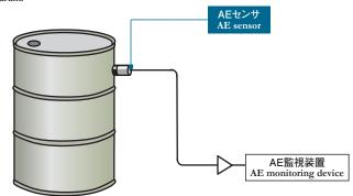
AE sensors can pick up warning signals from manufactured products that human senses cannot detect.
